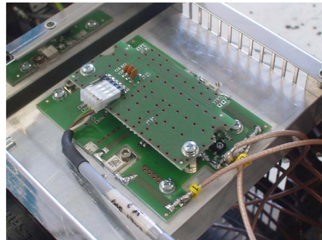
Exciter RF switch
